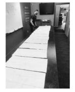
A pleated media filter, like those manufactured by Aprilaire or Amana, provides less restriction to airflow. This is accomplished by increasing the amount of surface area that the air must pass through by using many pleats or folds. When fully stretched out, an Aprilaire 16 x 20 filter has about 19 feet of media as shown in photo to the left.
